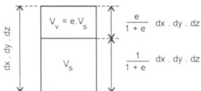
$$\frac{\partial}{\partial t} = \frac{\partial}{\partial t} \left( \frac{e}{1+e} dx dy dz \right) = \frac{\partial e}{\partial t} \times \frac{dx dy dz}{1+e}$$
