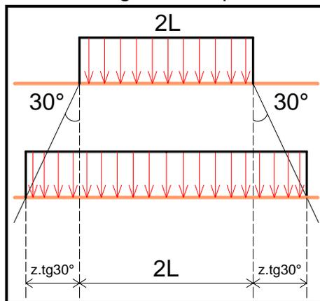
$$\sigma_v = \sigma_0 \times \frac{2 \times L}{2 \times L + 2 \times z \times \text{tg} 30^\circ}$$
